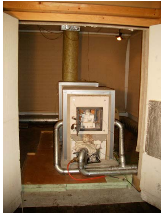
Figure 3: Experimental appliance in calorimetric chamber for measurements
